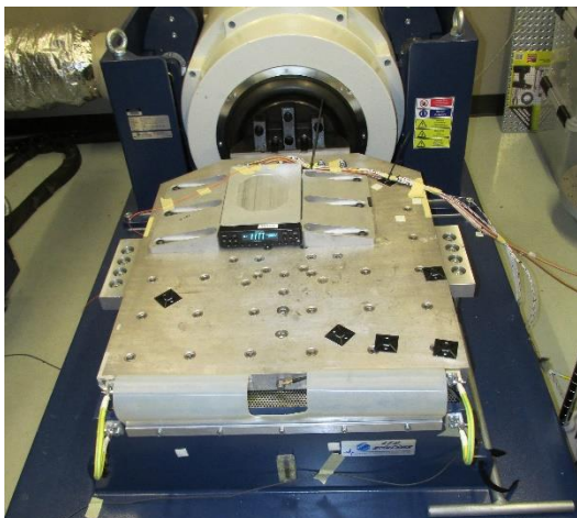
Device mounted on shaker table for testing
